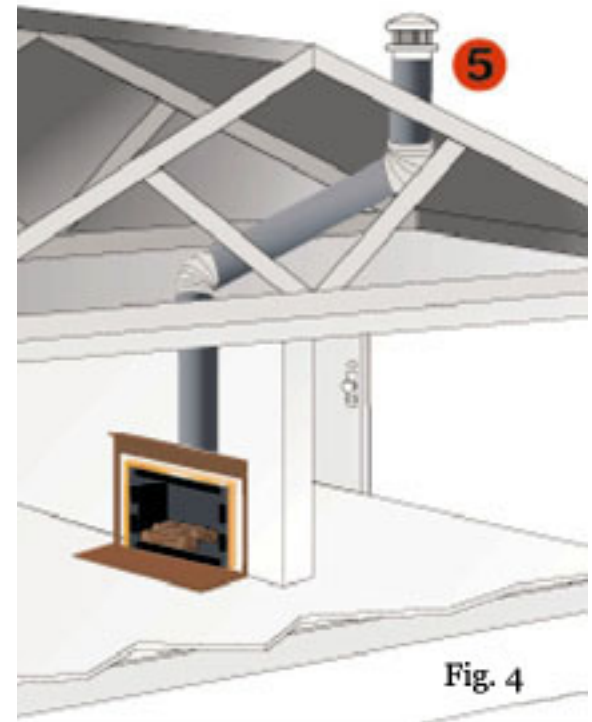
Fig. 4 Chimney offsets can be implicated in smoke spillage
